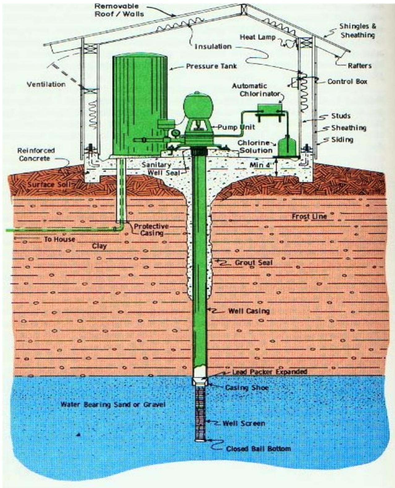
**Diagram 4:** Pump Housing – From USEPA Manual of Individual Water Supply Systems
