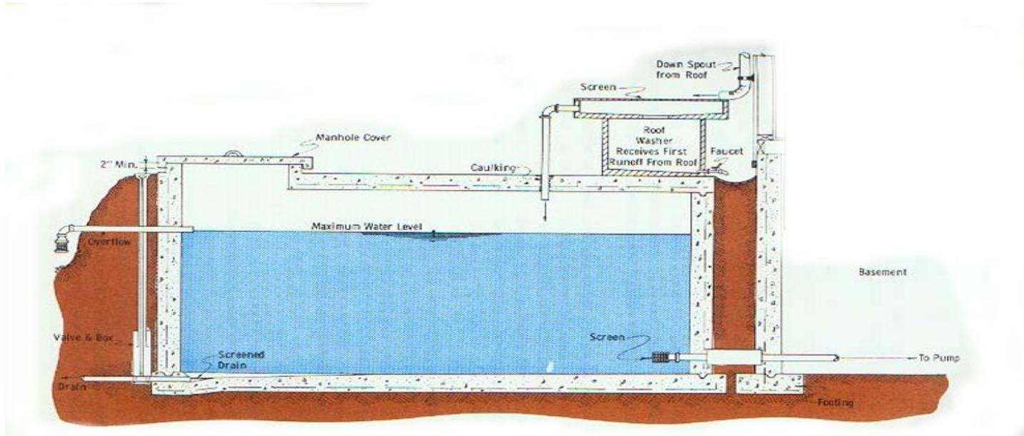
**Diagram 3: Cistern and trap cross-section**
