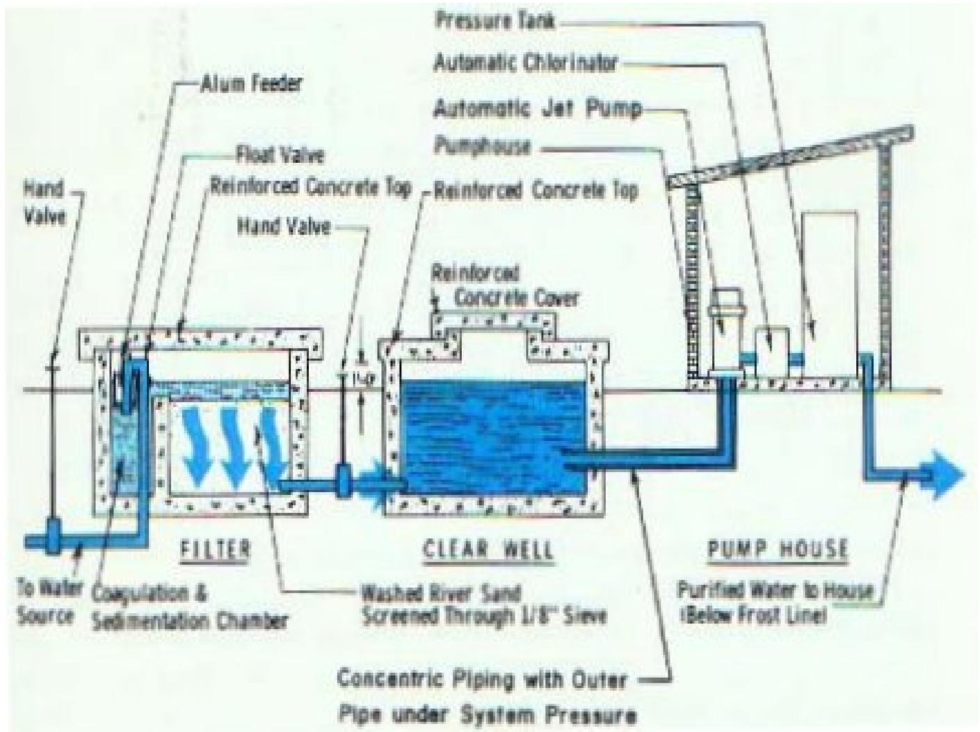
**Diagram 2: Pond Filter - From USEPA Manual of individual Water Supply Systems**
